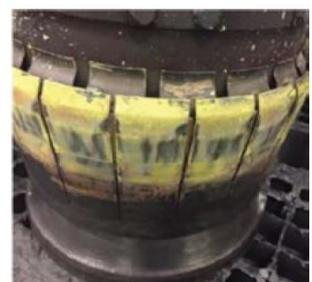
4. GT combustor basket spring clips showing deposit of hexavalent chromium
